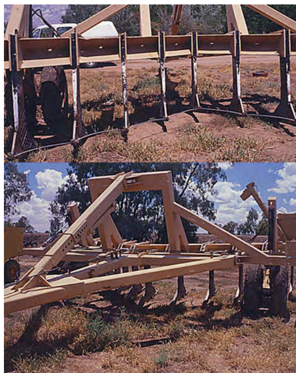
A trailing ripper set up for heavy cultivation of nutgrass after picking. Note the steel cable across the rippers (top photo) designed to cut the nutgrass roots during ripping.
