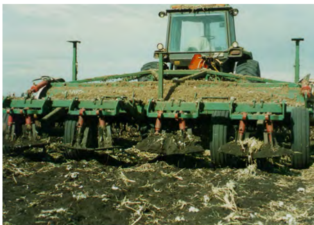
Always remember to clean off machinery like this root cutter before moving the machinery to different areas. This will help to prevent the spread of weeds. Photo: Greg Salmond.
