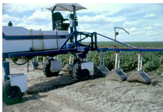
A purpose-built, high clearance sprayer set up for shielded spraying.
