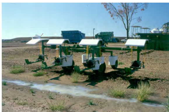
A purpose-built, spot-spraying rig set up for four operators, spraying weeds in 8 rows at a time.
