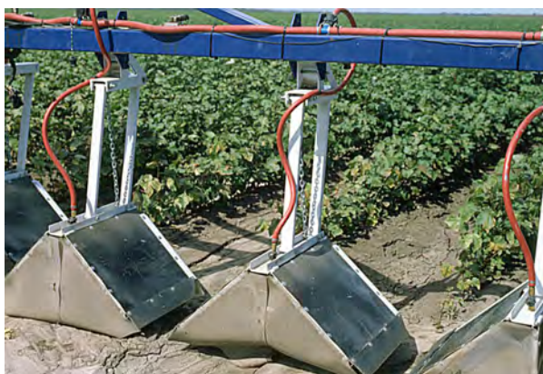
Glyphosate can be applied through spray shields to the area between the cotton rows in conventional cotton varieties. The spray shields prevent the herbicide contacting the foliage of the crop.
