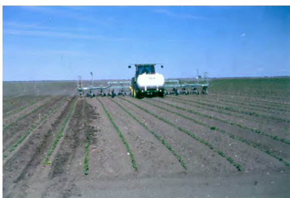
Inter-row cultivation can be used through the season to control weeds in the inter-row area and to maintain irrigation hills. Herbicides and fertiliser may also be applied through the cultivation rig.
