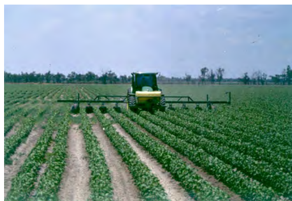
A purpose-built shielded sprayer being used to inter-row spray a troublesome weed, polymeria takeall, in young cotton.
