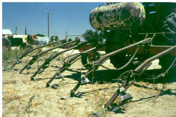
A homemade flame weeder for controlling weeds in the inter-row area. Not too much has to go wrong before this unit would set the tractor alight!
