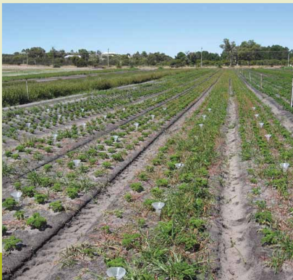
Catch cans setup in beds of parsley, at Natoli Produce Farms, to assess distribution uniformity of sprinkler system.
