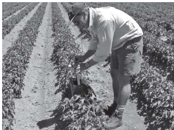
New Cotton CRC Farming Systems Scientist, Dirk Richards (CSIRO), measures soil moisture with a neutron probe
