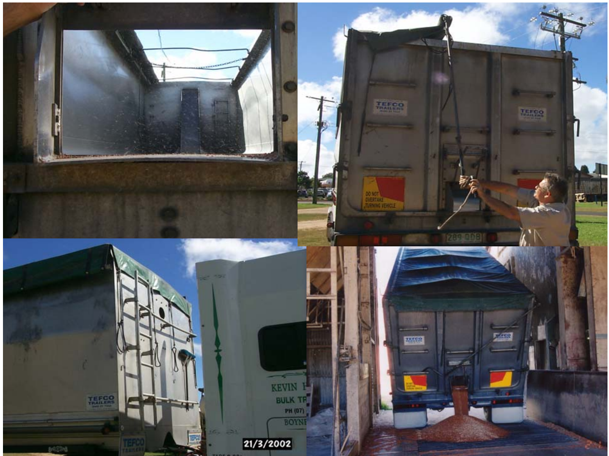
Photo 1a (upper left) Trailer floor moulded to the side walls prevents seed escape. Photo 1b (upper right) and Photo 1c (lower left) Fitting of the tarp does not allow over-filling of the trailer. Photo 1d (lower right) The chute, allows for accurate unloading.
