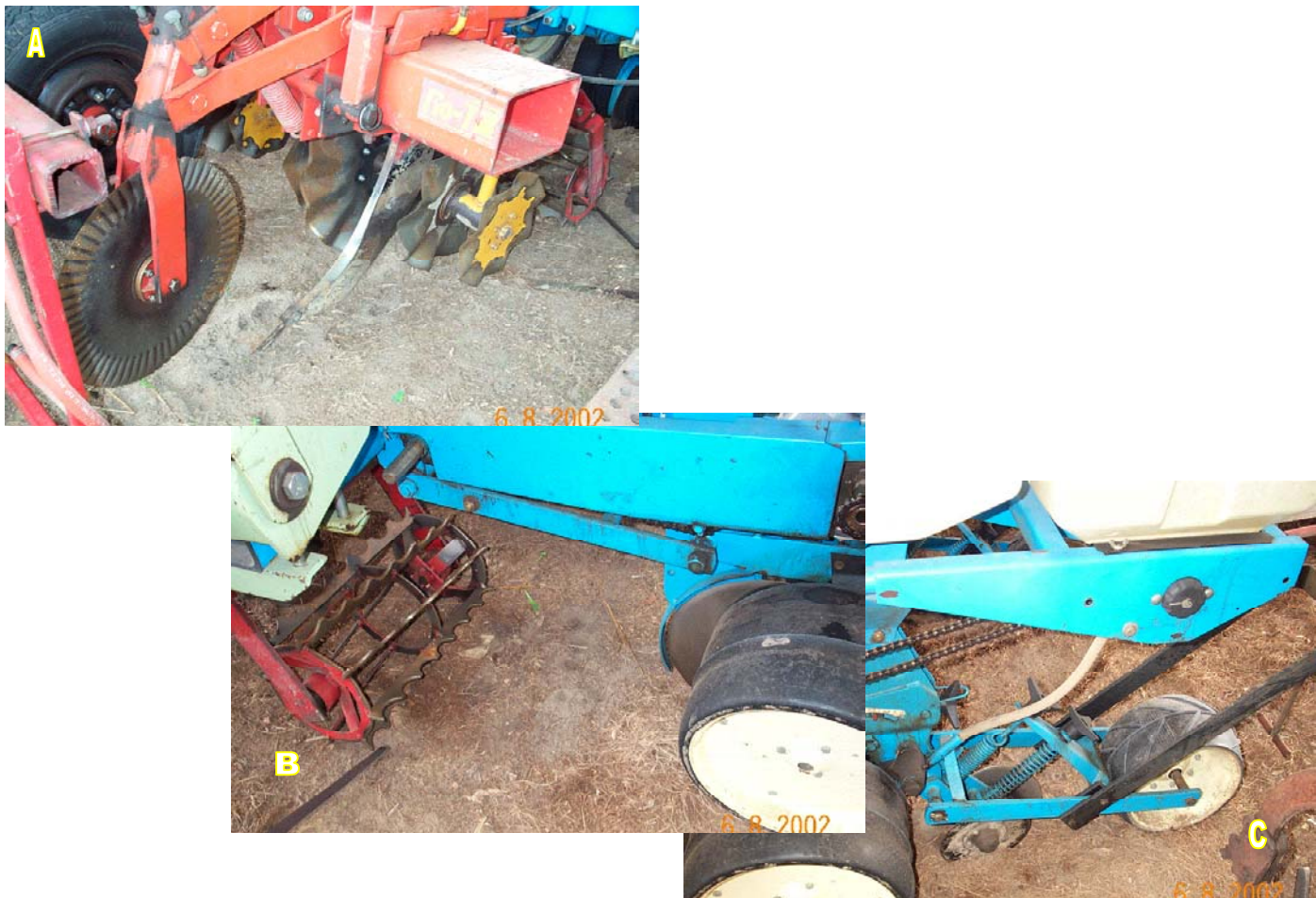
Plate 10: Strip till planter, A) coulter, ripping tyne, coulter for tilled band B) harrow, C) disc planter + presswheels.
