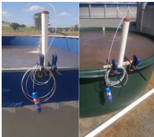
Figure 18: Odyssey's capacitance water level sensor probe and the PVC shroud installed in the evaporation ponds and water troughs. (Photograph: A. Leung)
