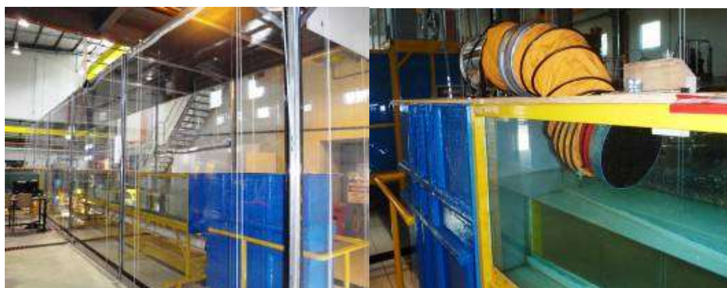
Figure 10: The wind and wave tank set-up showing the external structure enclosing the tank and the blower situated above the water surface. (Photograph: P. Schouten).
