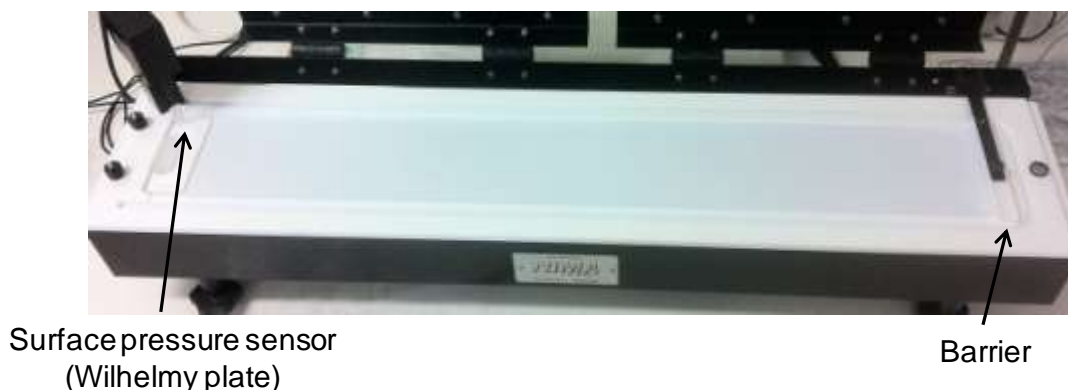
Figure 3: Langmuir trough—apparatus commonly used for investigating monolayer properties. (Photograph: E. Prime)
