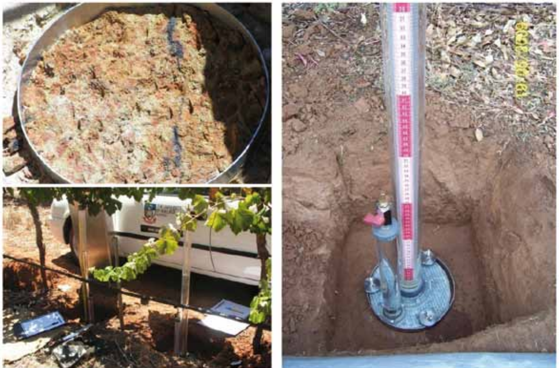
Infiltration rate measurement (clockwise from top left): a subsoil surface prepared for measurement, levelled permeameter in place ready to commence measurement, simultaneous measurements underway directly beneath and mid-way between well-spaced (2 metres) drippers.
