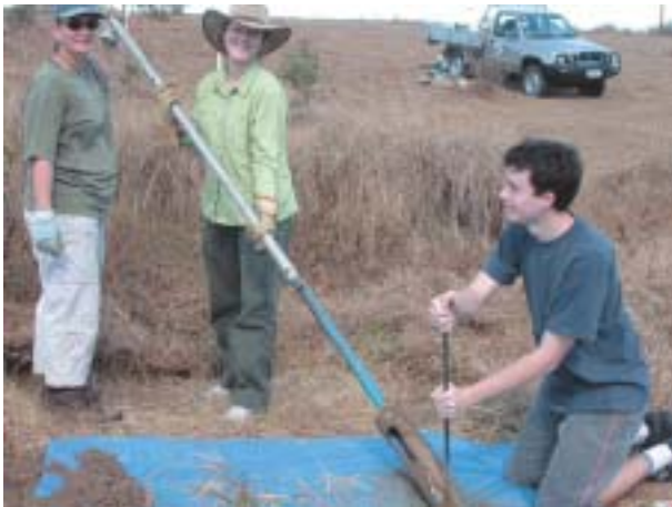
Collecting soil samples for denitrification potential measurements. Photo Carol Conway.
