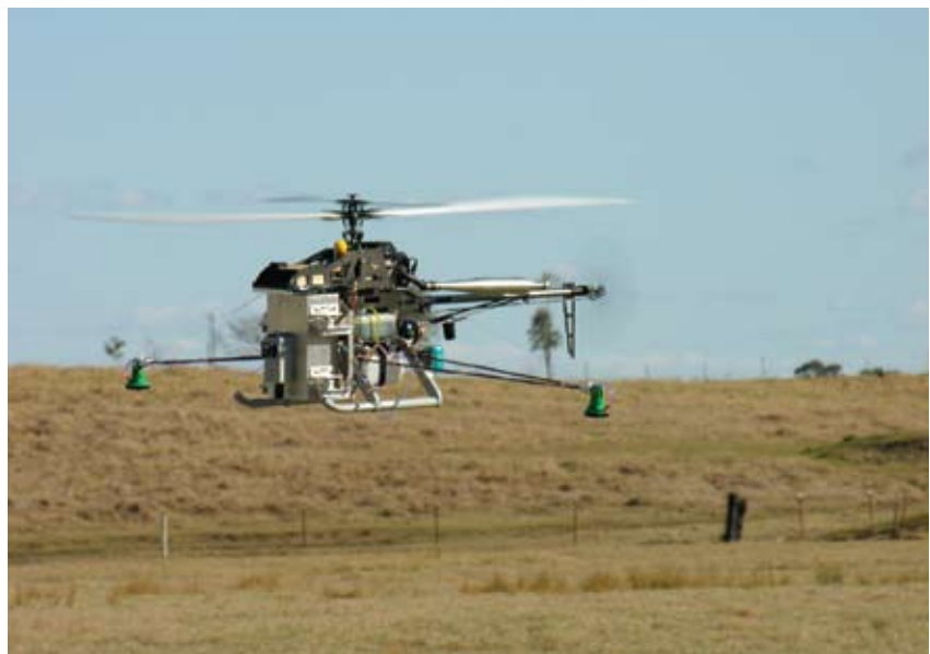
1. A photo of the aerial robot. The aluminium casing at the front of the robot houses the computer processing and imaging sensors. The two boom arms and spray module deliver the spray (water in these tests) to the desired location. Photo by Muhammad Esa Attia
