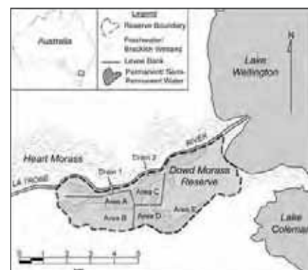
Figure 2.3: Dowd Morass, showing the location on internal levees and the resultant division of the wetland into five discrete zones.
