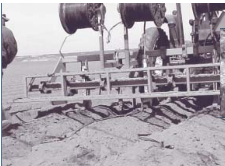
Laying of buried drip tape on the surface of raised vegetable beds, Santa Maria, California.
