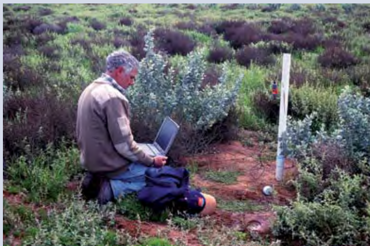
Department of Agriculture Technical Officer Meir Altman downloading a data logger attached to a continuous water level recorder. The loggers are notoriously fickle - we often lose the data - which may explain the "prayer like attitude"!
