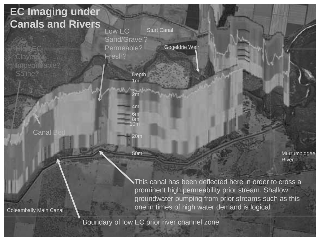
Figure 12.5 EC imagery collected using a floating geoelectric array towed along the Coleambally Main Canal (funding provided by the Rice CRC).
