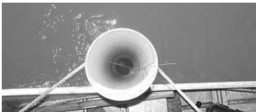
Figure 12.3 A SPOT. Note that the water level was originally at the level of the ‘hook’ on the wire in the tube and has fallen over a period of a few days while the canal level remained approximately constant.
