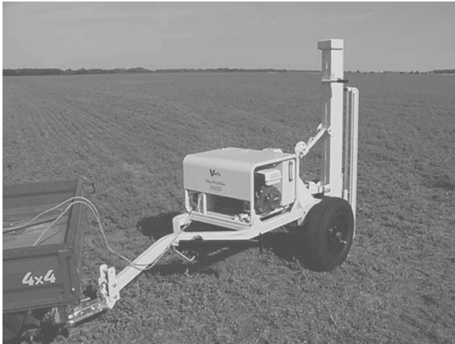
Figure 8.4 Veris Penetrometer with EC and pressure sensors.
