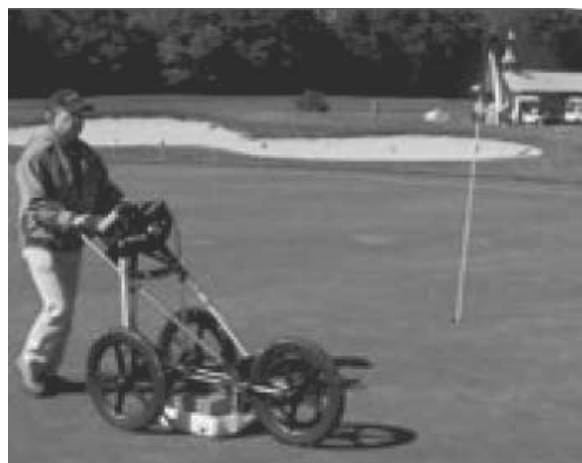
Figure 9.7 GSSI ground penetrating radar being used to identify soil structure variation
