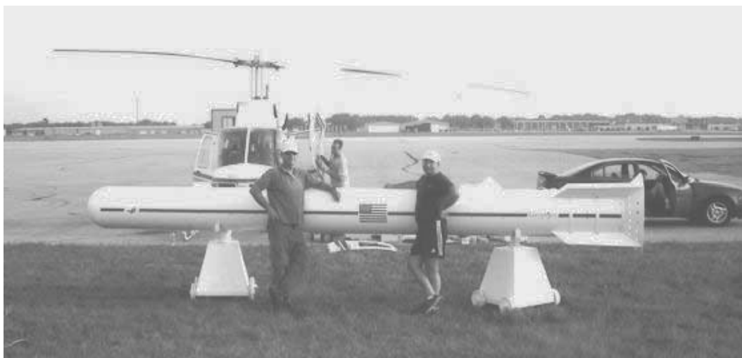
Figure 5.4 The GEM 2A broadband FDEM device weighing only 110 kg.
