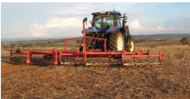
A rolling prickler harrow bar used to knock down stubbles and improve the decomposition potential for soil microbes.
